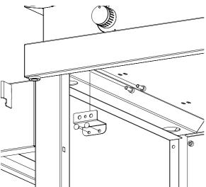
CAUTION do not break the 4 knockouts on the sides of the doors.
