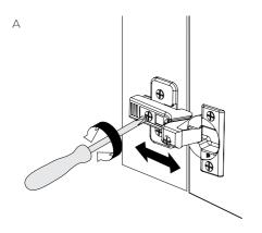
Adjust the doors as shown in images  ${\bf A}$ ,  ${\bf B}$ , and  ${\bf C}$ .
