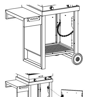
When using the trolley to house a cylinder, fit the safety chain to hold the cylinder firmly in place.
